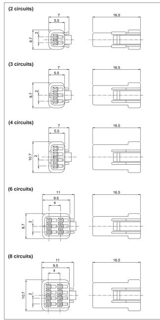
Note: Housing comes with seal rubber plate.
