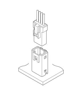
This JWPF connector can be used for the place of which especially waterproof is reauired.
