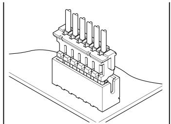
The ZH connector is very small with a mounting height of 5.6mm and a thickness of only 3.5mm. Contact retention lances on the housing make insertion easier, while the dimple at the center of the contact ensures reliable contact with the post.
