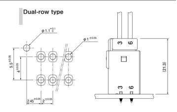
Note: 1. The above figure is the figure viewed from the connector mounting side.
