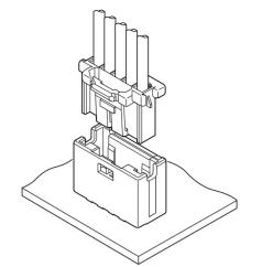
This connector is 2.5mm pitch wire-to-board connector that has a mechanism to prevent an incomplete mating by utilizing the inertial force when mating connector.
