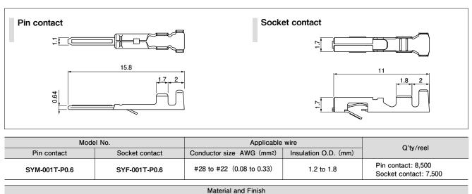
Pin contact: Phosphor bronze, tin-plated Socket contact: Phosphor bronze, tin-plated
