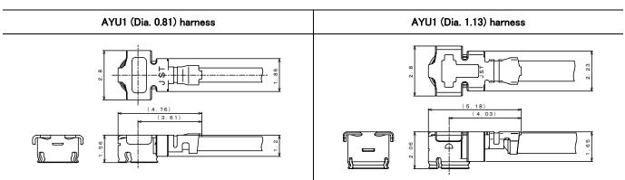
Material and finish Contact: Copper alloy. Nickel-undercoated, gold-plated. Housing: Thermoplastic resin, UL94V-0
