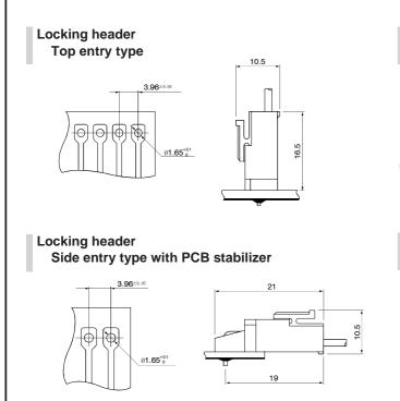
Note: 1. The above figure is the figure viewed from soldering side.
