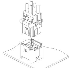
This HYV connector is 5.0 mm pitch wireto-board type connector and has the mechanism to supperss the incomplete mating in mating operation.
