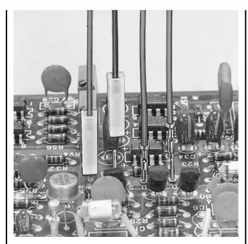
This small single-circuit connector connects to 1.0mm and 1.3mm diameter pins and requires only minimal space for connection of wires to high-density printed circuit boards.
