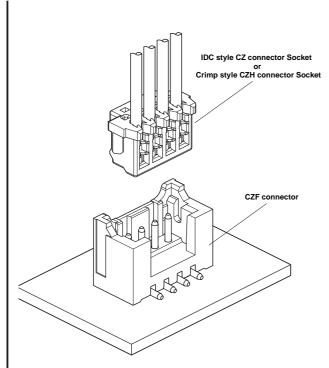
The SMT top entry type headers that can be mated with the 1.5 mm pitch CZ connector socket are on the lineup.
