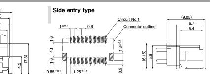
Note: 1. The above figure is the figure viewed from the connector mounting side. 2. Tolerances are non-cumulative: ± 0.1 mm for all centers. The dimensions above should serve as a guideline. Contact JST for details.
