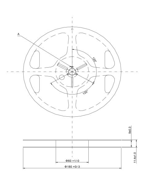
Material:Polystyrene (Conductivity) unit:mm
