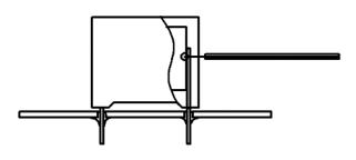
Temperature monitored inside the capacitor.
