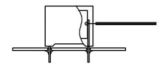
Temperature monitored inside the capacitor.
