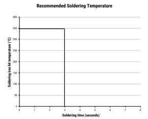
Soldering iron tip temperature should be set at 350°C (+10°C maximum), with the soldering duration not to exceed 3 seconds.
