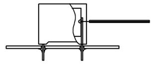
Temperature monitored inside the capacitor.
