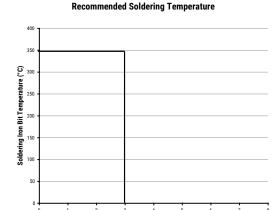
Soldering iron tip temperature should be set at 350°C (+10°C maximum), with the soldering duration not to exceed more than 3 seconds.
