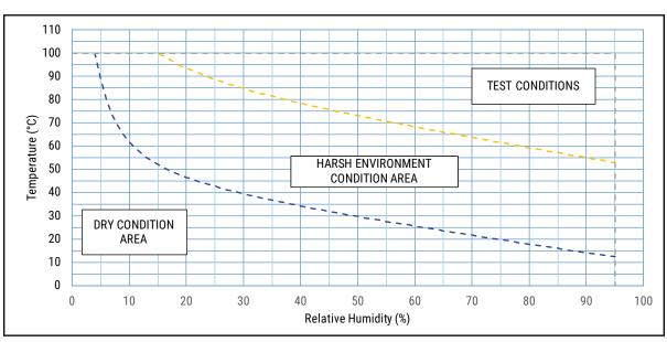
The dry condition area is defined as the range of temperature and relative humidity to validate the life time and  $V_{rms}/I_{rms}$  graphs. The separation line between harsh environment conditions and test conditions area is calculated for a life time of one year at operating voltage.
