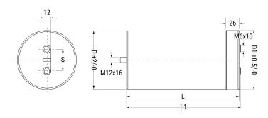
General Information Series C44U-M Dielectric Metallized Polypropylene Style Features DC Filtering, Energy Storage RoHS With Exemptions **REACH** SVHC (Pb - CAS 7439-92-1) SCIP Number cc1c1ec4-db9e-4815-b26b-e8a34ddfb776 Screw Terminals M6 Lead AEC-Q200 Nο Component 1120 g Weight Thermal Resistance = 5.1 C/W. Weight = 5600 Miscellaneous grams.
