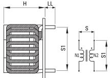
General InformationSeriesSC-JHStyleThrough-HoleRoHSYesNotesLead Spacing (S/S1) Are For Reference Only.MiscellaneousTemperature Rise Maximum: 50 KCoreMn-Zn Ferrite
