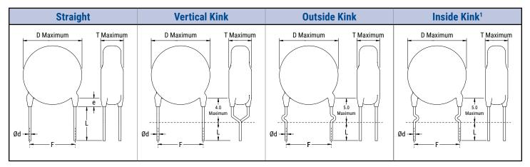
All lead configurations are available on devices with lead spacing of 10 mm and 12.5 mm.
