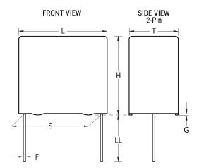
**General Information** Series F462 Dielectric Metallized Polypropylene Style Radial MKP, Pulse Features RoHS Yes Lead Wire Leads AEC-Q200 No Component 5.303 g Weight The Rated Voltage Decreases 2%/C Between +85C And +105C (1.25%/C For AC). ClimCat: Miscellaneous 55/105/56.
