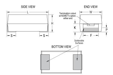
Series T409 CWR09 MnO2 Tantalum Dielectric Style SMD Chip Description SMD, MnO2, Molded, Military Equivalent RoHS No MARNING: Cancer and reproductive harm -Prop 65 http://www.p65warnings.ca.gov. Termination Solder Coated Qualifications MIL-PRF-55365/4, CWR09 Style AEC-Q200 No Component 349.01 mg Weight Note: When Option C Is Selected For Lead Material, Notes Add An Additional 0.38mm To The Tolerances For "L", "W", "H", "K", "F" And "S". MSL 1
