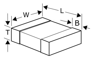
**General Information** Series VE Туре Varistors Style SMD Chip Description Surface Mount Varistors Features Low Voltage High Temperature Termination Nickel Tin RoHS Yes Qualifications IEC, UL, AEC-Q200 AEC-Q200 Yes
