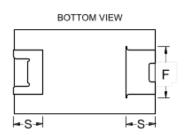
**General Information** Series T523 Dielectric Polymer Tantalum Style SMD Chip Description SMD, Polymer, Molded, Face Down Terminals Features Face Down RoHS Yes Termination Nickel Palladium Gold AEC-Q200 No **Component Weight** 274.3 mg 52 Weeks Shelf Life MSL 3
