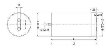
General Information Series C44U-M Dielectric Metallized Polypropylene Style Features DC Filtering, Energy Storage RoHS With Exemptions **REACH** SVHC (Pb - CAS 7439-92-1) SCIP Number cc1c1ec4-db9e-4815-b26b-e8a34ddfb776 Screw Terminals M6 Lead AEC-Q200 No Component 880 g Weight Thermal Resistance = 7.1 C/W. Weight = 4400 Miscellaneous grams.
