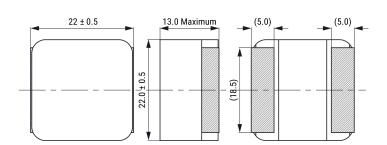
**General Information** Series MPXV Style SMD Chip Size 2213(9088) Description Surface Mount Inductor Features Power Inductors RoHS Yes Qualifications AEC-Q200 AEC-Q200 Yes Core Composite 40 (K) Temperature Rise Max. Miscellaneous
