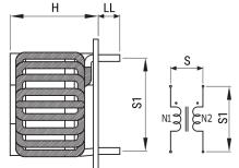
General InformationSeriesSC-JHStyleThrough-HoleRoHSYesNotesLead Spacing (S/S1) Are For Reference Only.MiscellaneousTemperature Rise Maximum: 75 KCoreMn-Zn Ferrite
