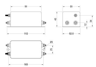
**General Information** Series FLLE2-P Style **Chassis Mount** Description Single Phase, Chassis Mount Filters Single Phase Features Phase Single-phase RoHS Yes Qualifications IEC/EN 60939, UL, CSA Threaded Studs M4 **Terminal Type**
