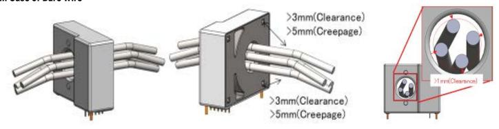
Reinforced insulation, insulation material group III, pollution degree 2, altitude < 5,000 m and overvoltage category II. Please take enough creepage distance between each pin.
