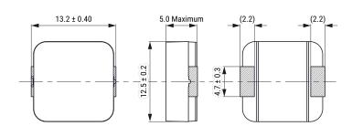
**General Information** Series MPXV Style SMD Chip Size 1250(5350) Description Surface Mount Inductor Features Power Inductors RoHS Yes Qualifications AEC-Q200 AEC-Q200 Yes Core Composite 40 (K) Temperature Rise Max. Miscellaneous
