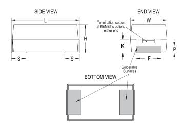
General Information Series T409 CWR09 Dielectric MnO2 Tantalum Style SMD Chip Description SMD, MnO2, Molded, Military Equivalent RoHS Yes Termination Gold Qualifications MIL-PRF-55365/4, CWR09 Style AEC-Q200 No Component 39.91 mg Weight Note: When Option C Is Selected For Lead Notes Material, Add An Additional 0.38mm To The Tolerances For "L", "W", "H", "K", "F" And "S". MSL 1
