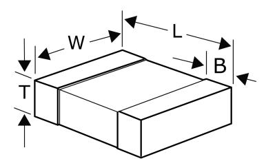
Series VC Туре Varistors Style SMD Chip Description Surface Mount Varistors Features Low Voltage Termination Nickel Tin RoHS Yes Qualifications IEC, UL, AEC-Q200 AEC-Q200 Yes
