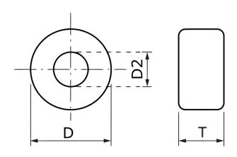
General Information Series ESD-R Style Round - Toroidal Cable Type Round Cable EMI Core Solid, For Round Cables, Toroidal Cores, Description Bare Type RoHS Yes UL94 V-2 Qualifications Materials Ni-Zn
