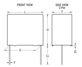
**General Information** Series PFR/F411 Dielectric Film/Foil Polypropylene Style Radial Features Pulse RoHS Yes Lead Wire Leads AEC-Q200 No Component 0.426 g Weight An Operating Temperature Up To +105C Is Miscellaneous Allowed Under Certain Conditions. Please Consult KEMET For Details.
