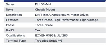
**Specifications** 530 VAC, 305 VAC Voltage AC 50-60 Hz Rated Frequency Rated Current 75 A (50°C) Rated Temperature 50°C Temperature Range -25/+100°C Climate Category 25/100/21 Test Voltage DC (P to P) 2250 VDC Test Voltage DC (P to E) 3000 VDC 30 W (25°C 50 Hz) Power Loss Leakage Current 4.7 mA
