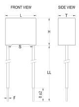
Dielectric Metallized Polypropylene Style Radial **EMI** Safety Features RoHS Yes Lead Insulated Flexible Leads Safety Class X2 ENEC, UL, cUL, CQC Qualifications AEC-Q200 No **THB** Performance No **Component Weight** 5.4 g
