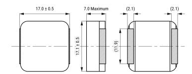
**General Information** Series MPX Style SMD Chip Size 1770(6868) Description Surface Mount Inductor Features Power Inductors **RoHS** Yes Core Composite Miscellaneous 40 (K) Temperature Rise Max.
