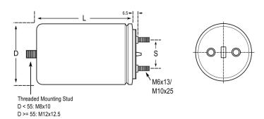
General Information Series C44A Dielectric Metallized Polypropylene Style Can RoHS With Exemptions **REACH** SVHC (Pb - CAS 7439-92-1) SCIP Number cc1c1ec4-db9e-4815-b26b-e8a34ddfb776 Lead Threaded Studs M6 AEC-Q200 No Component Weight 148.3 g Thermal Resistance = 7.8 C/W. Miscellaneous
