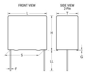
**General Information** Series F612 Dielectric Metallized Polyester Style Radial MKT (Stacked), DC Multipurpose Applications Features RoHS Yes Lead Cut/Short AEC-Q200 No Component 0.23 g Weight The Rated Voltage Decreases 1.25%/C Between +85C And +105C (For +125C, Please Consult Miscellaneous Kemet). This 5% tolerance part is available on request. ClimCat: 55/105/56.
