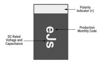
DC Rated Voltage and Capacitance Code
