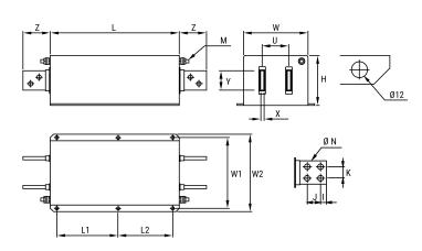
**General Information** Series FLLE2-PV Style Chassis Mount Description EMI Filter, Without Y Capacitor Single Phase, Photovoltaic Applications Features Phase Single-phase RoHS Yes Qualifications IEC/EN 60939, UL 1283 Threaded Studs M16 **Terminal Type**
