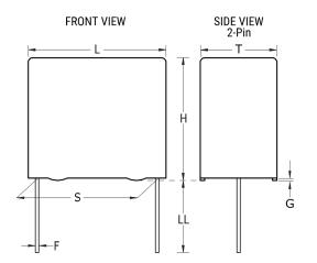
**General Information** Series F461 Dielectric Metallized Polypropylene Style Radial MKP, Pulse Features RoHS Yes Lead Wire Leads AEC-Q200 No Component 0.379 g Weight The Rated Voltage Decreases 2%/C Between +85C And +105C (1.25%/C For AC). ClimCat: Miscellaneous 55/105/56.
