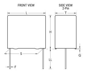
**General Information** Series F461 Dielectric Metallized Polypropylene Style Radial MKP, Pulse Features RoHS Yes Lead Wire Leads AEC-Q200 No Component 0.378 g Weight The Rated Voltage Decreases 2%/C Between +85C And +105C (1.25%/C For AC). ClimCat: Miscellaneous 55/105/56.
