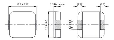
Series MPX Style SMD Chip Size 1235(5350) Description Surface Mount Inductor Features Power Inductors **RoHS** Yes Core Composite Miscellaneous 40 (K) Temperature Rise Max.
