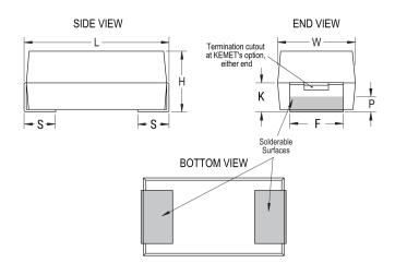
MnO2 Tantalum Dielectric Style SMD Chip Description SMD, MnO2, Molded, Military Equivalent RoHS No 🛕 WARNING: Cancer and reproductive harm – Prop 65 http://www.p65warnings.ca.gov. SCIP Number 1dd2e1b8-26dd-4d52-927c-6f9d519011aa Termination Solder Coated Qualifications MIL-PRF-55365/4, CWR09 Style AEC-Q200 No Component 349.01 mg Weight Note: When Option C Is Selected For Lead Notes Material, Add An Additional 0.38mm To The Tolerances For "L", "W", "H", "K", "F" And "S". MSL 1
