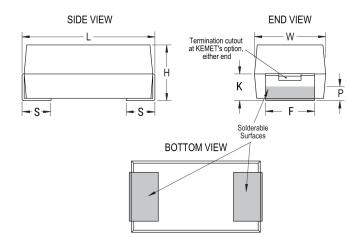
Series T492 CWR11 MnO2 Tantalum Dielectric Style SMD Chip Description SMD, MnO2, Molded, Military Equivalent RoHS No 🛕 WARNING: Cancer and reproductive harm -Prop 65 http://www.p65warnings.ca.gov. SCIP Number 1dd2e1b8-26dd-4d52-927c-6f9d519011aa Termination Solder Coated Qualifications MIL-PRF-55365/8, CWR11 Style AEC-Q200 No Component 412.33 mg Weight Note: When Option C Is Selected For Lead Notes Material, Add An Additional 0.38mm To The Tolerances For "L", "W", "H", "K" ,"F" And "S". MSL 1
