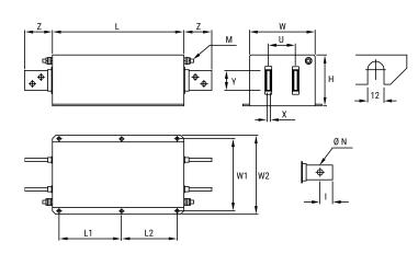
**General Information** Series FLLE2-PV Style Chassis Mount Description EMI Filter, With Y Capacitor Single Phase, Photovoltaic Applications Features Phase Single-phase RoHS Yes Qualifications IEC/EN 60939, UL 1283 Threaded Studs M10 **Terminal Type**
