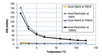
Temperature dependencies of ESR measured at 10 kHz and 100 kHz for Axial Hybrid (PHA225MKP3370QE1) and Axial Electrolytic (PEG226MG3370QE1) capacitors.
