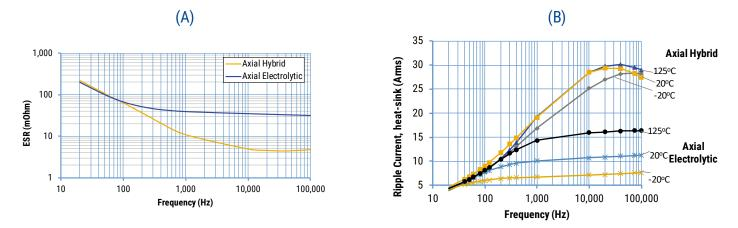
Frequency dependencies of ESR measured at 20°C and 100 kHz for Axial Hybrid (PHA225MKP3370QE1) and Axial Electrolytic (PEG226MG3370QE1) capacitors (A); Frequency dependencies of max. short pulse Ripple Current at different temperatures for heat-sink mounted Axial Hybrid (PHA225MKP3370QE1) and Axial Electrolytic (PEG226MG3370QE1) capacitors (B).
