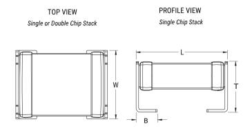
General Information Series KPS SMD Comm X7R Style Stacked Chip SMD, MLCC, Stacked, Single Chip, Temperature Description Stable Features Temperature Stable RoHS Yes Termination Tin AEC-Q200 No Component 170 mg Weight 1812-1 Chip Size Shelf Life 78 Weeks MSL 1
