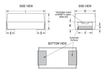
General Information Series T409 CWR09 MnO2 Tantalum Dielectric Style SMD Chip Description SMD, MnO2, Molded, Military Equivalent RoHS Yes Termination Gold Qualifications MIL-PRF-55365/4, CWR09 Style AEC-Q200 No Component 68.73 mg Weight Note: When Option C Is Selected For Lead Notes Material, Add An Additional 0.38mm To The Tolerances For "L", "W", "H", "K", "F" And "S". MSL 1
